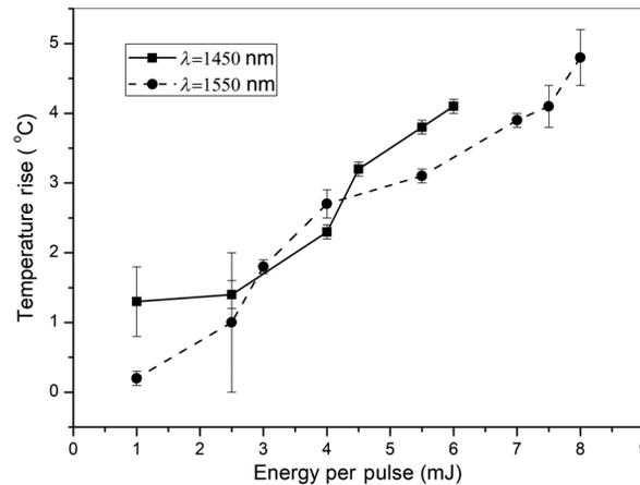
**Fig. 4** The variation of temperature induced by different energy per pulse. Pulse duration is 18 ms and repetition rate is 9.5 Hz.
