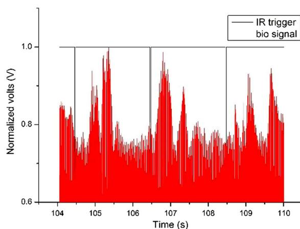
**Fig. 6** Variation of measured voltage after laser pulse. The black line indicates the location of onset laser irradiation (the repetition rate of laser is 2 Hz).
