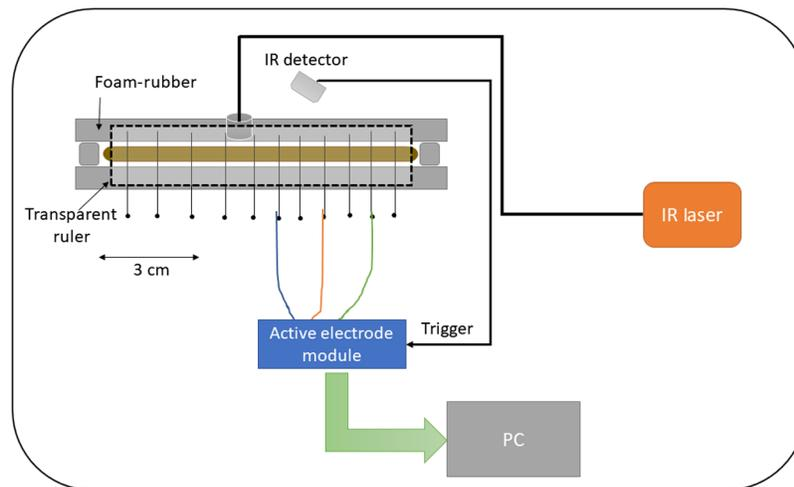
**Fig. 1** The cage keeping earthworm. The laser light is delivered to worm via a 200- $\mu\text{m}$  multimode optical fiber. An IR amplified detector (PDA20H, Thorlabs) is used to trigger the active electrode module.
