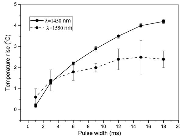
**Fig. 3** The effects of pulse duration on the temperature. The repetition rate is 9.5 Hz and energy per pulse for 1450 and 1550 nm are 6 and 8 mJ, respectively.
