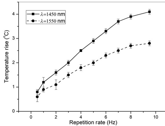
**Fig. 2** Variation of temperature for two different wavelengths of 1450 and 1550 nm versus the repetition rate. Pulse duration is 18 ms and energy per pulse for 1450 and 1550 nm are 5 and 6 mJ, respectively.
