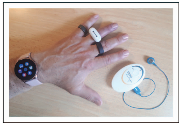
FIGURE 2. A demonstration of a variety of wearables on one hand. The hand demonstrates, from thumb onwards has the Circul, Sleepoon, and Oura ring attached, a Smartwatch with PPG, Photoplethysmography recording and a sleep analyser app, and the M1 Sleepimage device next to the hand to be attached on the chest. My own camera with my own hand (Thomas Penzel).
